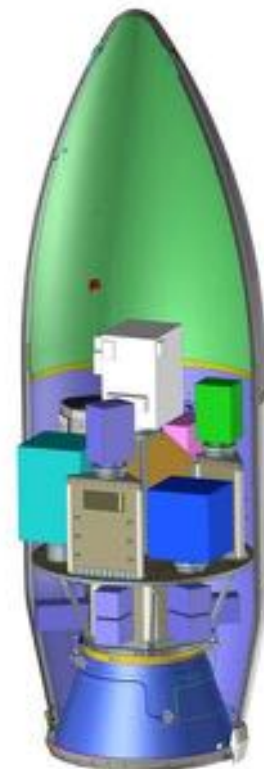
SSMS/Avumw orbital kit for releasing sats at different inclination/altitu
